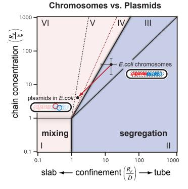
FIG. 5 Chromosome vs. plasmid. The two axes represent confinement ( $x = R_F/D$ ) and chain concentration ( $y = R_F/\xi$ ). For *E. coli* B/r (H266), we estimated x = 13.6 and y = 37.5 for the chromosome. Plasmids correspond to approximately one order of magnitude smaller values of x and y (see text).
