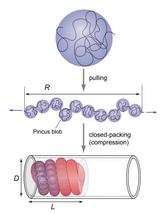
FIG. 2 In the scaling theory, stretching of a self-avoiding chain can be mapped onto compression of the chain via closed-packing into a confined space using the concept of blob. The compression free energy of the chain obtained this way is consistent with the results obtained by seemingly different methods Jun *et al.* (2007); Sakaue and Raphaël (2006).
